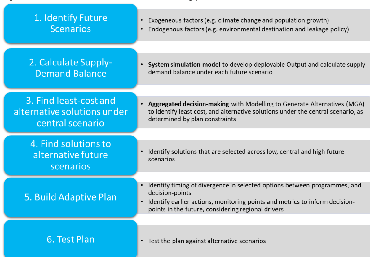
Figure 3-3: Schematic of WRMP decision-making process
