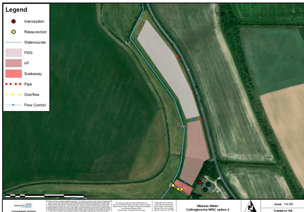
Figure 8 - Collingbourne Ducis WRC wetlands layout - Option 2 (area required to meet the performance target)
