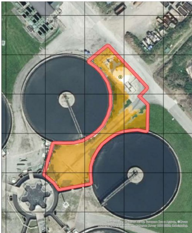
Figure 5 – Avonmouth Sludge Import Reception Bund
