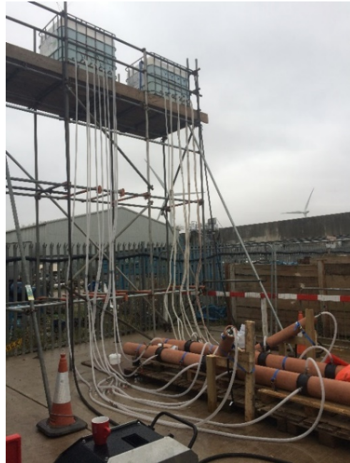
Figure 3-6: Test rig for epoxy lining trials using new resin technology
