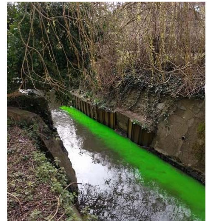
Dye test showing foul sewer interacting with the river 2017
