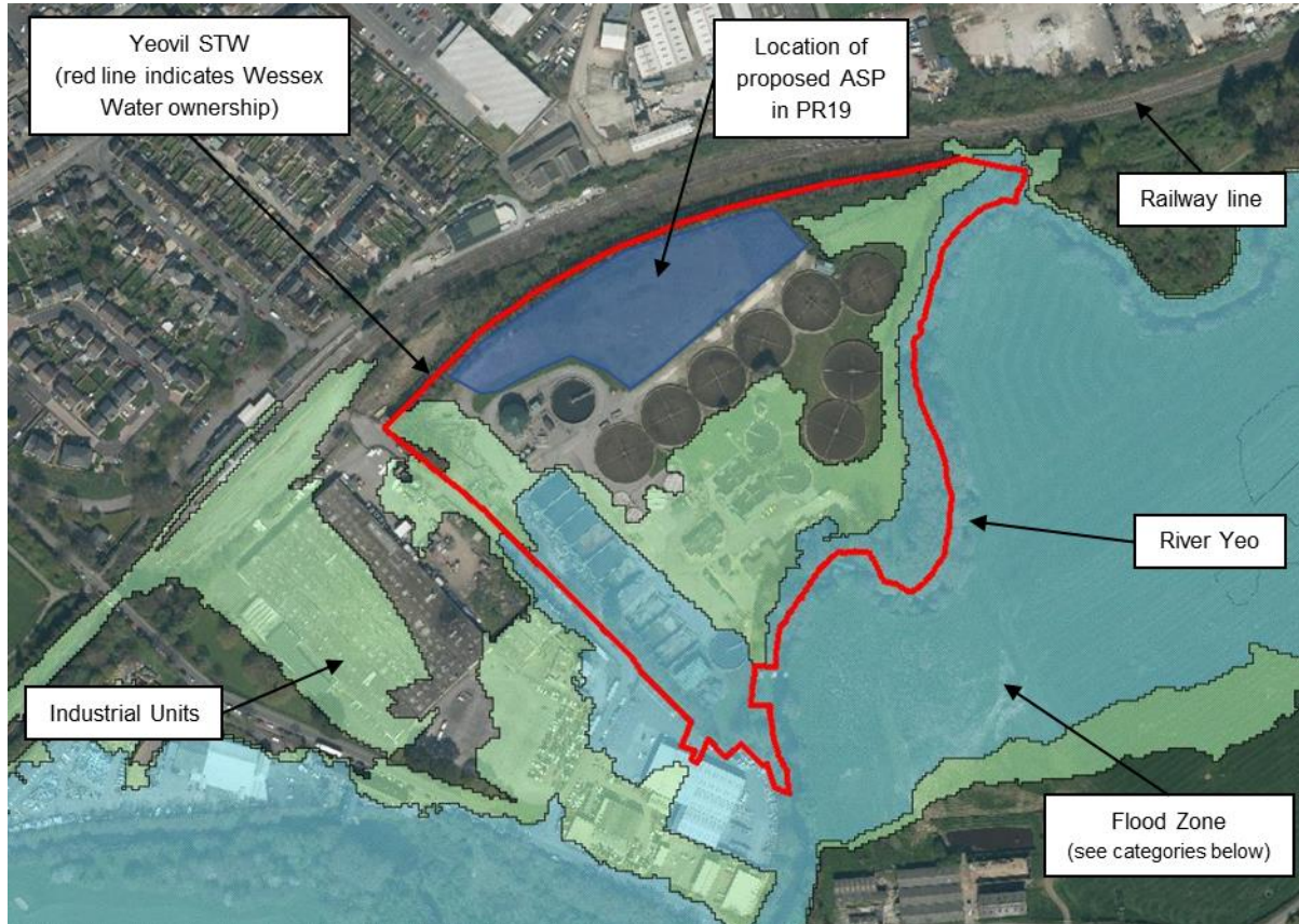
Figure H-1: Site plan of Yeovil (Pen Mill) STW showing constraints to future expansion
