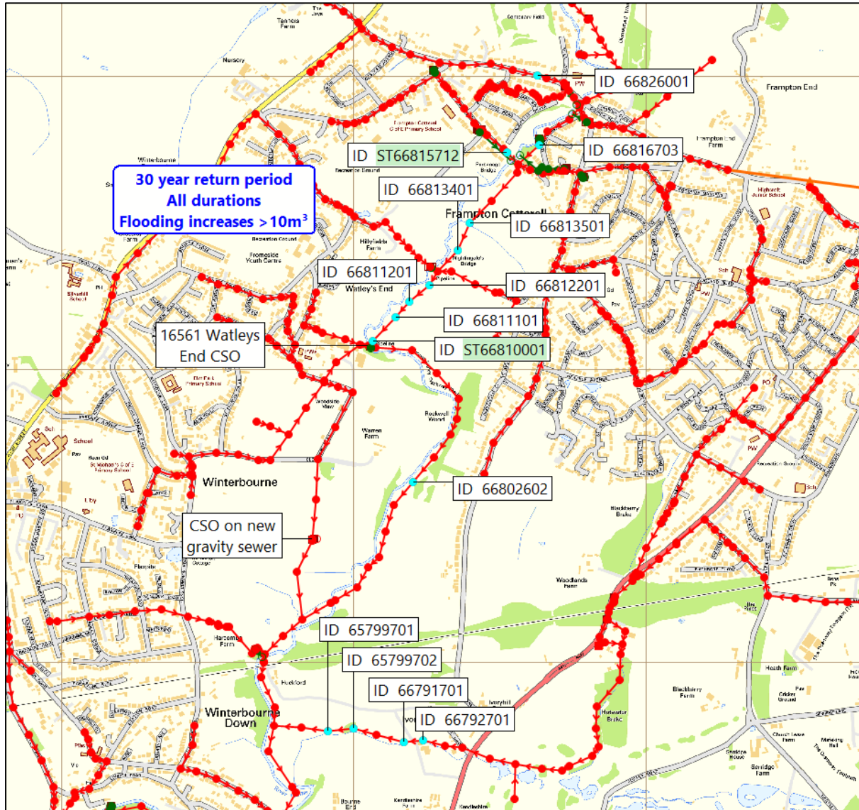
Option 2 – manholes where flooding is predicted to increase >10m³ for 30-year return period
